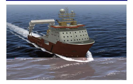
The K-Sim Engine Offshore Krupp MaK M42 AHTS model is based on a medium speed Engine Room configuration from a modern Anchor Handler, Tug & Supply vessel (AHTS) carrier with 4 Krupp Mak medium speed engines and 2 x controllable pitch in fixed kort nozzles. The model has 1 x 2040 Bhp tunnel & 1 x 1770 Bhp CP Retractable Azimuth as the forward thrusters and 2 x1200 BHP tunnel Stern thrusters.
